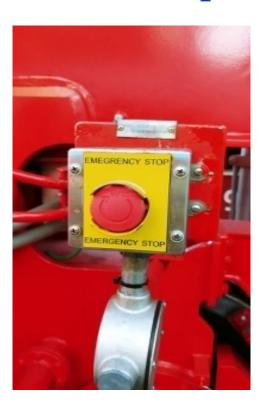
We should all be aware that ship to shore cranes, container yard rubber-tired gantry cranes and container yard rail-mounted gantry cranes are typically fitted out with one or more emergency stop buttons that can be accessed at ground level..
